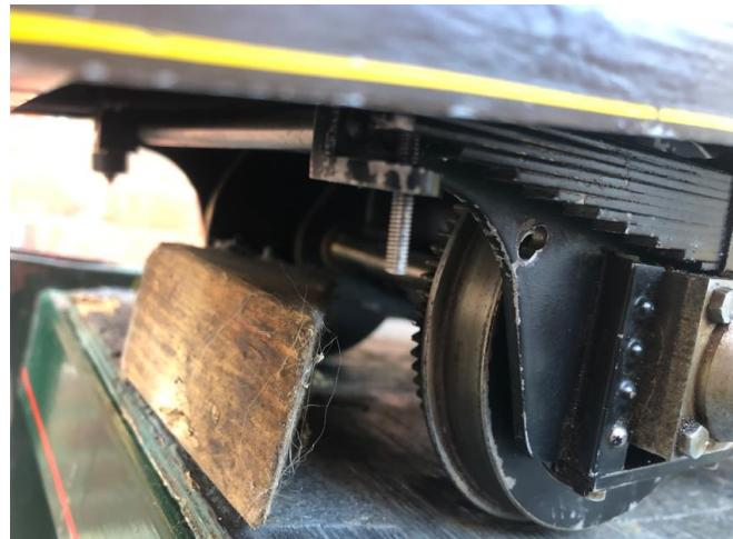
It was at this point I noticed various nuts and bolts were loose and one part on the end of a dummy spring had gone altogether!
