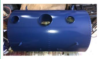
Earlier this month the boiler passed its 1½ times working pressure hydraulic test.
