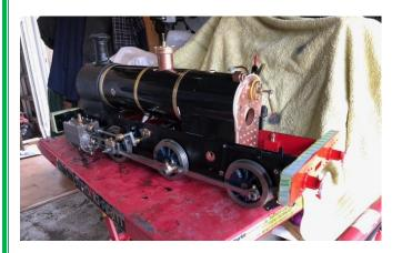
The cladding is now attached and the boiler fitted into the frames.
