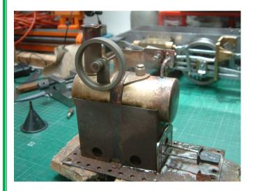
After the successful first steaming the engine was completely disassembled and cleaned, polished and re-painted. The paint used was the same as my 3 ½" Tich which I knew stuck well to the substrate metal and took the heat of a steam engine. Phoenix Precision two pack etch primer was used followed by synthetic enamel topcoat all applied by airbrush.
