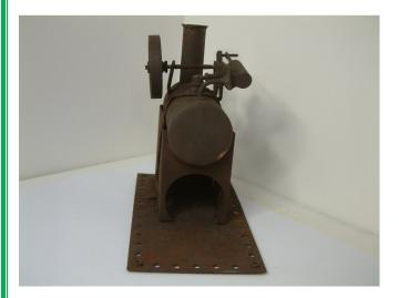
The engine was taken apart and cleaned, oiled, boiler tested, pipe between the boiler and the cylinder re-soldered, safety valve un-seized and serviced and the engine re-assembled and tested on compressed air at about 5 to 10 PSI, it ran beautifully. The engine was then put into steam and ran really well, the crank and cylinder trunnion screw were a bit sloppy in the frames from use but this did not seem to affect the performance of the 70 year old engine.
