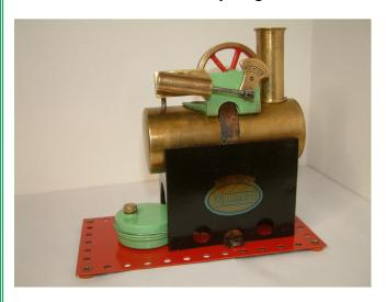
Now completed, the engine has been run regularly and operates with ease my Mamod WS1 Workshop which I saved up my pocket money and bought when I was 14. You can get 20 to 30 minutes of continuous running with one boiler and burner filling when using the glass fibre wick which does not burn down in use.
