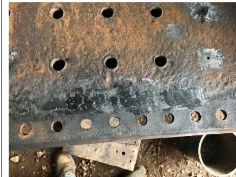
Figure 10 - First practice at building up pitting using the arc welder
