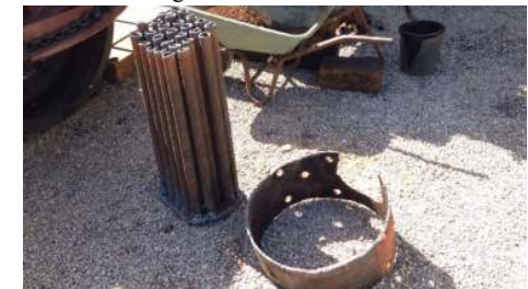
Figure 3 - Smokebox off and tube nest/tubes out
