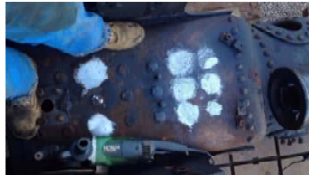
Figure 5 - Half way through grinding the crown stays
