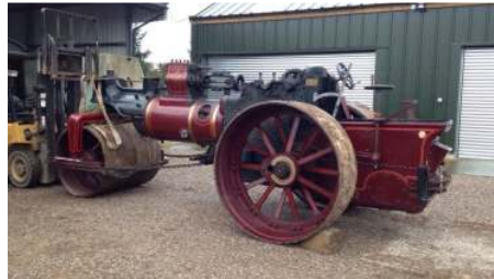
Figure 3 - Removing the front rolls from the headstock
