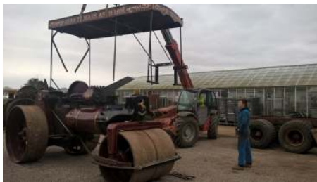
Figure 2 - We have lift off! Removing the canopy with the telehandler
