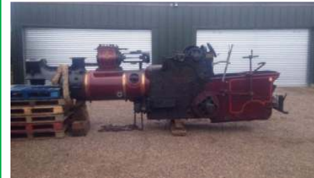
Figure 5 - Rear rolls removed
